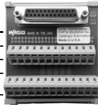
Figure 8 – A30/T4x-Series I/O Block
