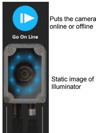
The Go Online puts the camera online or offline. When it is online, it will capture an image when a trigger input signal is received.
