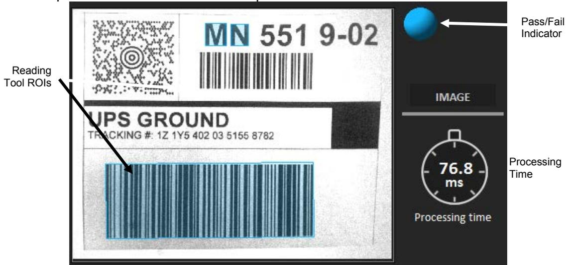
The Image window displays the image currently being inspected. Reading Tool ROIs turn red if a code or character tool read fails. The Pass/Fail Indicator turns red if any part of the inspection fails. Processing time includes the amount of time it takes for the camera to capture and inspect the image.
