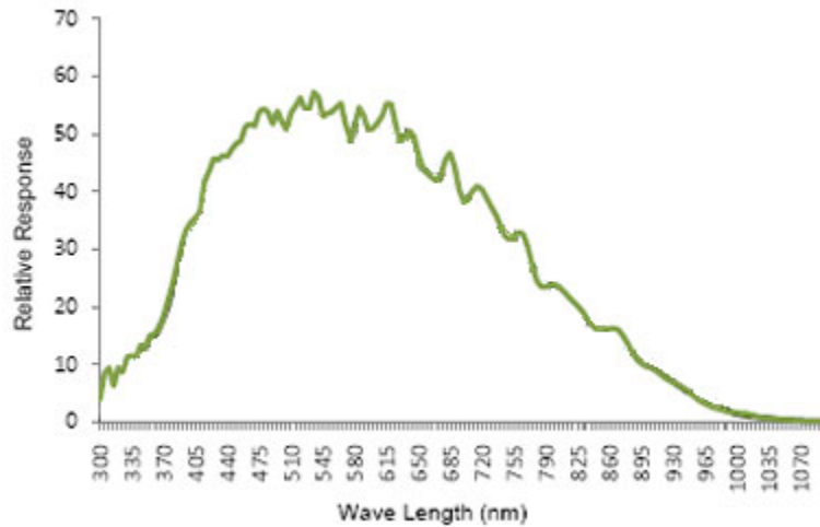
M190 Spectral Response (excludes lens and light source characteristics)
